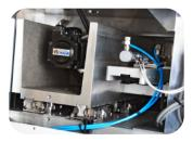
Heavy, cast aluminum-alloy frame provides the weight and rigidity required to absorb vibration and dissipate heat.
