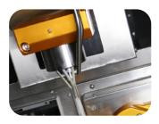
Powerful Spindle and Coolant Delivery.
